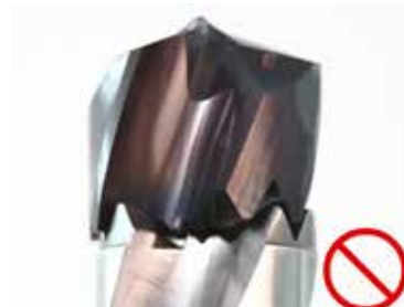
Chip flute and tooth profile do not line up
