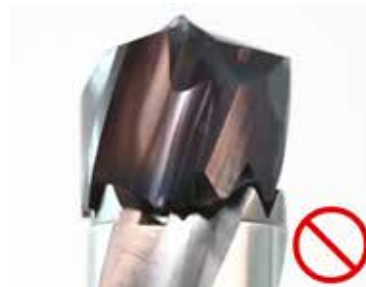
Chip flute and tooth profile do not line up
